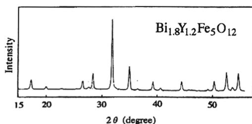
Fig.2 X-ray diffraction pattern of Bi-YIG particles.
