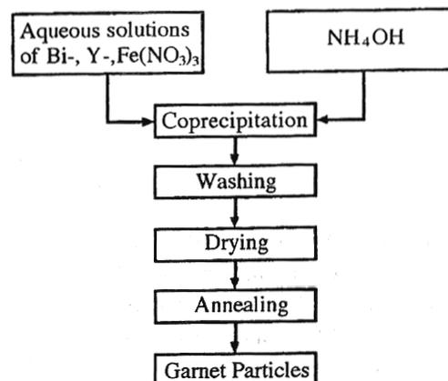
Fig.1 Preparation process of Bi-YIG particles by coprecipitation and annealing.
