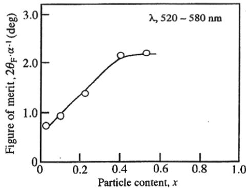
Fig. 9 The figure of merit of the Bi-YIG coated films in the visible wavelength region.
