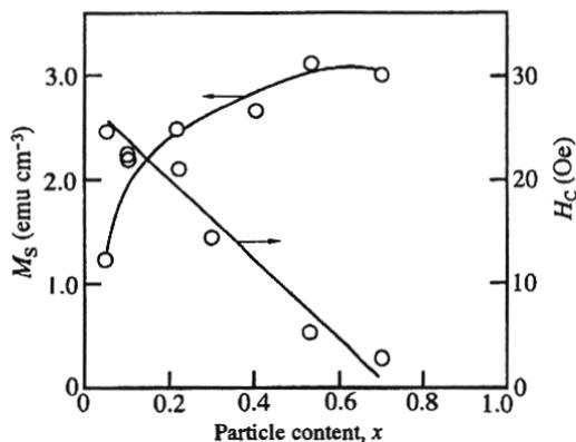
Fig.6 Saturation magnetization and coercive force of the films as a function of particle content  $x$ .
