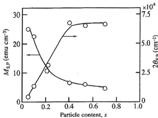
Fig. 8 Saturation magnetization and Faraday rotation expressed in units per particle volume in the films.
